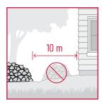
Remove combustible materials (firewood and lumber) stored within 10 m of house perimeter and under decks.
