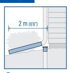
Disconnect downspouts, cap foundation drains and extend downspouts to direct water at least 2 m from foundation.
