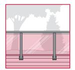
Retrofit all deck components to be fire-rated, with a continuous surface.
